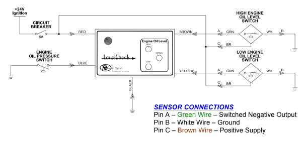
Caution: Damage will occur to the sensor if the connections are incorrect. This will void warranty.
